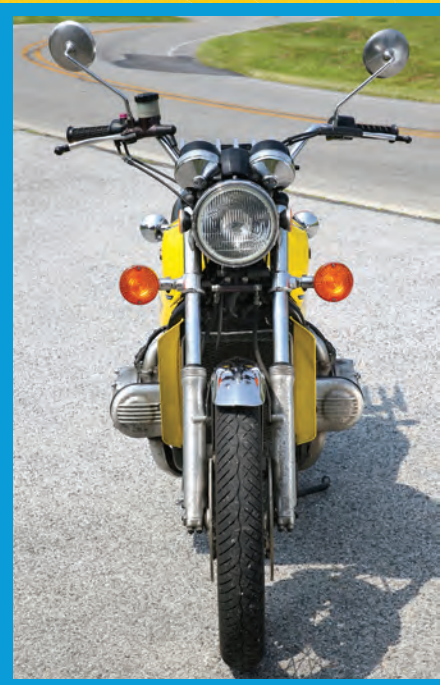
Left: Soichiro Honda thought the Gold Wing's horizontally opposed cylinders resembled a bat. Right: A low center of gravity contributes to the GL's good handling.
